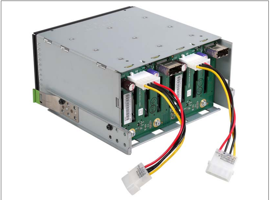
Figure 46: Connecting PS adapter cable to HDD backplanes
